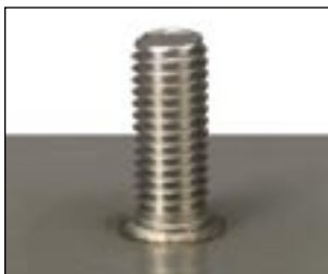
Small, regular and spatter-free collar
