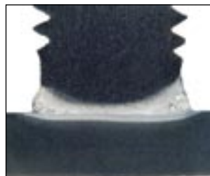
Narrow fusion zone. No arc blow effect
